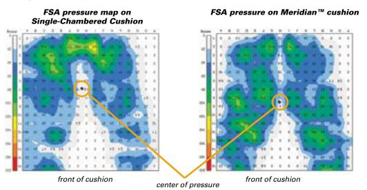
The Meridian cushion enables the client or caregiver to adjust the pelvic chamber independent of the thigh chamber. This allows maximum immersion of the pelvis, and pressure is redistributed off the ITs and onto the thighs.
