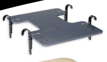
VARILITE Drop Base is made from durable and lightweight 3/8-inch (1 cm) PVC. Our L-J brackets are hardened steel for superior strength and durability. The hardware allows 4 inches (10 cm) of height adjustment and 15 degrees of angle adjustment-great for changing the seat-to-floor height or seat-to-back angle.
